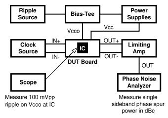
Figure 11-1. PSRR Test Setup
