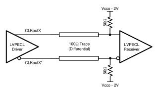
Figure 10-8. Differential LVPECL Operation, DC Coupling
