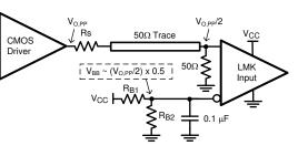
Figure 10-3. Single-Ended LVCMOS Input, DC Coupling with Common-Mode Biasing
